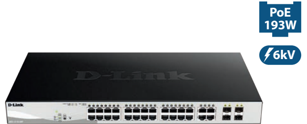
DGS-1210-28P/FL • 24 x 10/100/1000Base-T PoE ports Up to 193 W PoE power budget • 4 x 1000Base-T/SFP combo ports Dimensions: 440 x 250 x 44 mm
